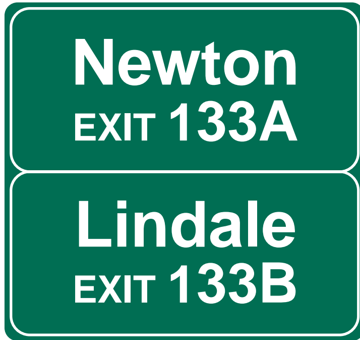
Figure 2E-15. Supplemental Guide Signs for Multi-Exit Interchanges
