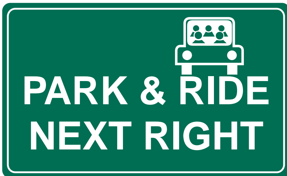
Figure 2-16. Supplemental Guide Sign for a Park and Ride Facility (Route without Exit Numbering)
